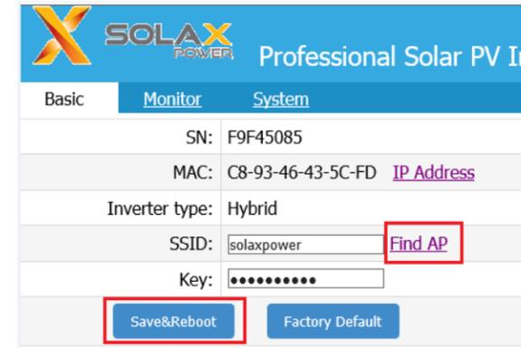
Click "Find AP" as shown below. There will be a scan page, it will search for the signal of WIFI router around. Signal means strength of the router. 100% means the router has a good signal, 0% means the router has no signal here.
