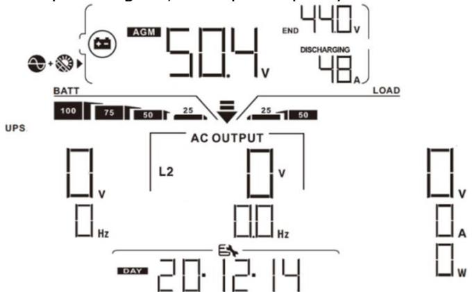
Output voltage, load in VA, load in Watt switch every 5 second/
