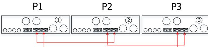
**WARNING:** Do not connect the current sharing cable between the inverters which are in different phases. Otherwise, it may damage the inverters.
