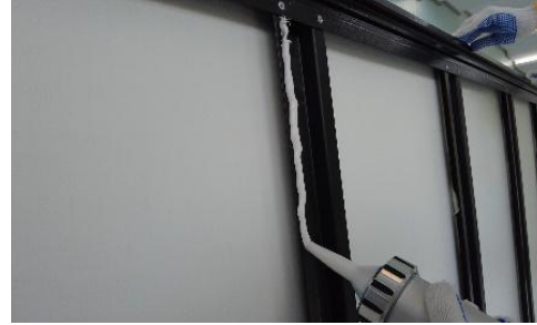
② Apply glue to the short side of the mounting structure
