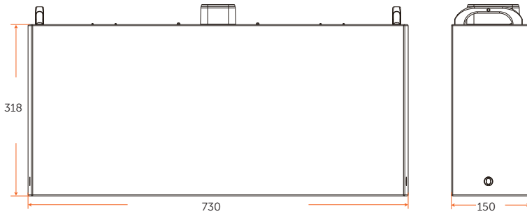
Figure 2-8 Dimension: Battery module (TP-HS50E)
