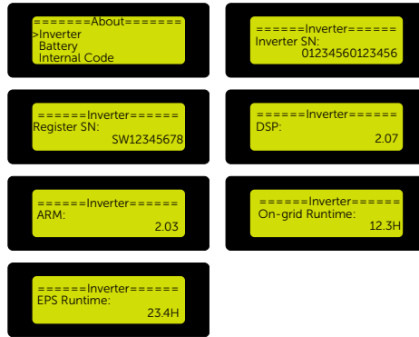
Figure 9-102 Displaying the inverter information
