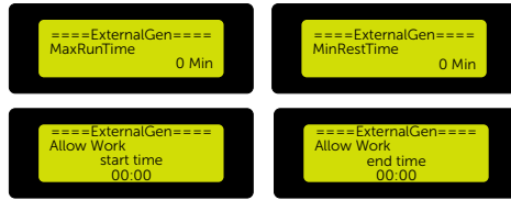
Figure 9-82 Setting MaxRunTime, MinRestTime, allow working period
