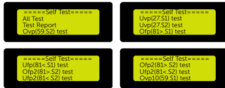
Figure 9-51 Setting to do tests
