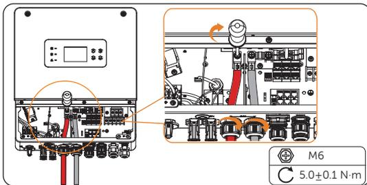
Figure 8-42 Tighten the cable
