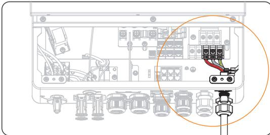
Figure 8-14 Grid cable connected
