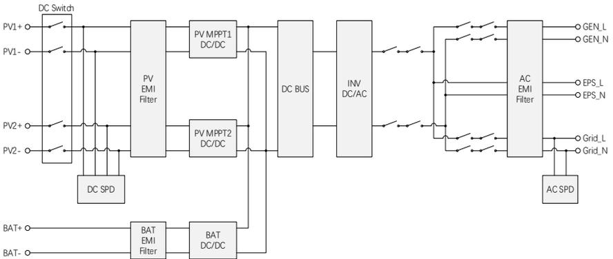
Figure 2-7 Circuit Diagram for X1-Hybrid-LV series inverter
