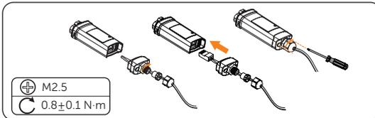
Figure 8-78 Assembling the LAN dongle
