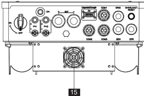
Figure 8-3 Terminals of Inverter (Bottom view 2)
