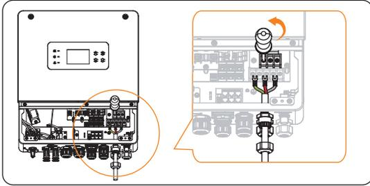
Figure 8-18 Insert the EPS cable
