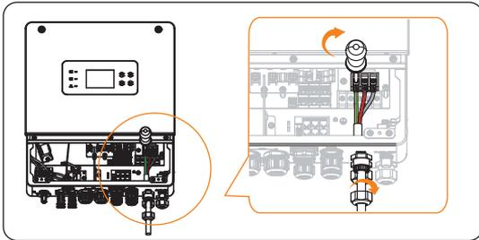
Figure 8-19 Tighten the EPS cable
