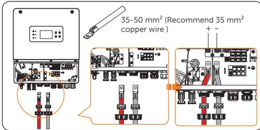
Figure 8-40 Pass and insert the cable
