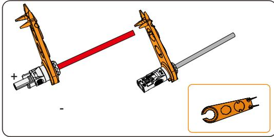
Figure 8-27 Loosening the swivel nut
