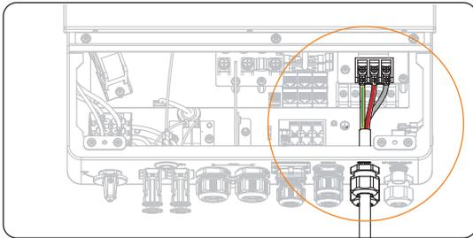
Figure 8-20 EPS cable connected
