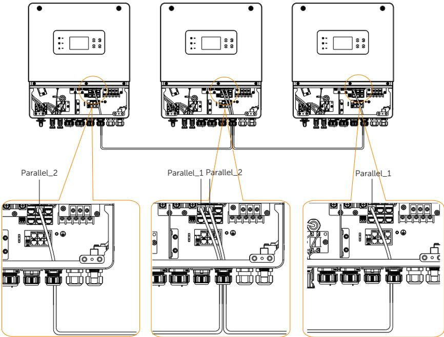
Figure 8-66 Parallel connection diagram
