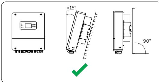
Figure 7-1 Correct installation
