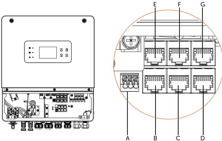
Figure 8-46 Communication ports
