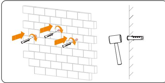
Figure 7-7 Insert the expansion tubes
