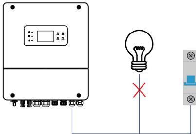
Figure 8-1 Wrong connection of load and inverter
