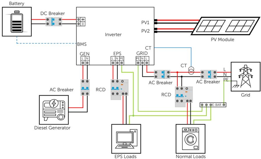
Figure 2-8 Wiring methods for most of the countries
