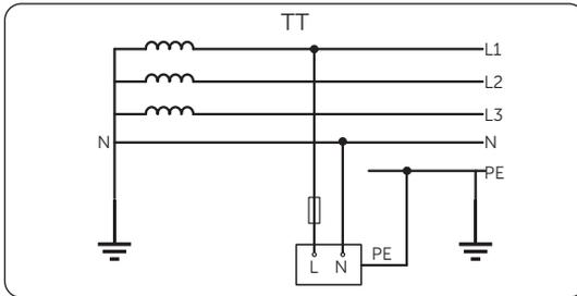
Figure 2-1 Supported power grid TT
