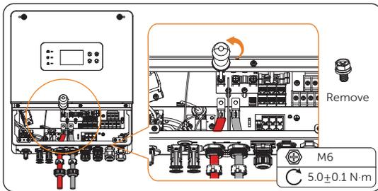
Figure 8-41 Remove the screw
