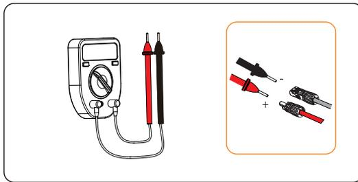
Figure 8-28 Measuring the voltage of PV connectors
