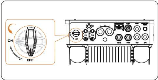
Figure 13-2 Turning off DC switch
