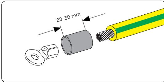
Figure 8-5 Installing the tubing and OT terminal
