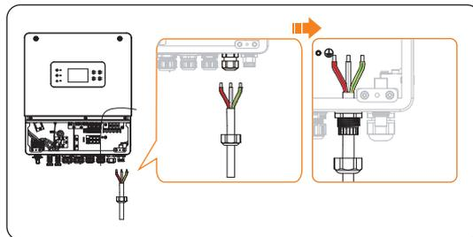
Figure 8-8 Pass the GEN cable
