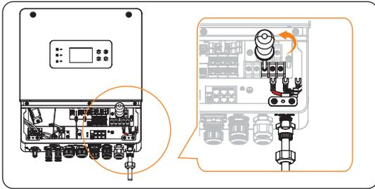
Figure 8-12 Insert the Grid cable
