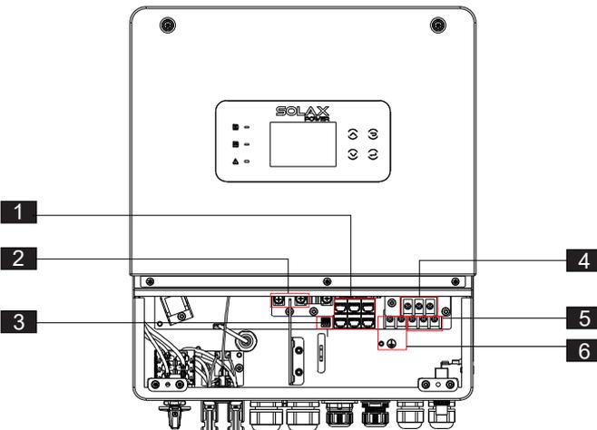
Figure 8-1 Terminals of Inverter (Front perspective view)
