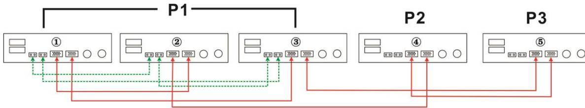
Two inverters in two phases and only one inverter for the remaining phase:
