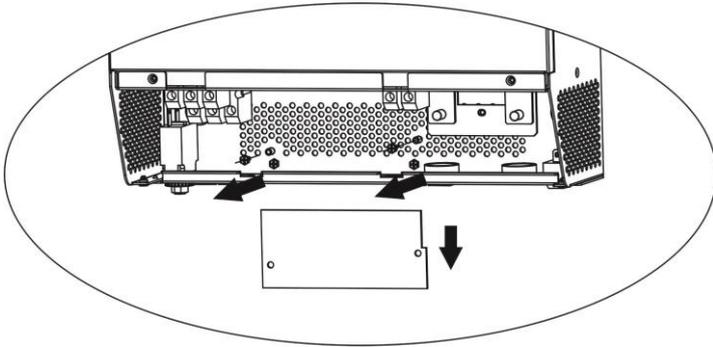
**Step 4:** Remove two screws as below chart to take out cover of parallel communication.
