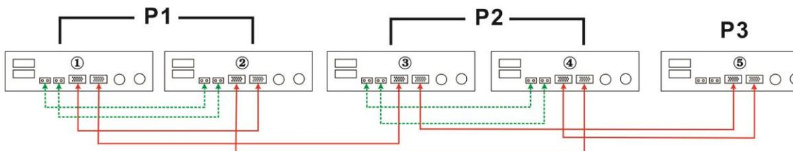
Two inverters in one phase and only one inverter for the remaining phases:
