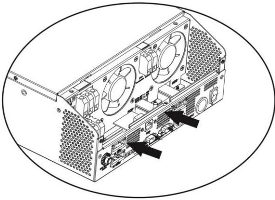
**Step 8:** Put wire cover back to the unit. Now the inverter is providing parallel operation function.
