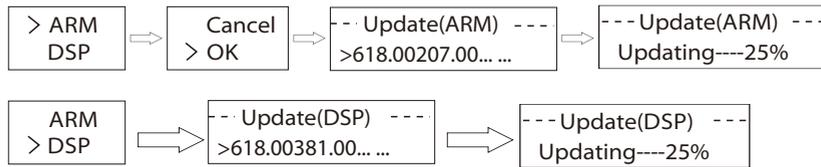
5) After the upgrade is complete, please remember to turn off the DC switch and the AC switch, then pull off the USB flash driver.
