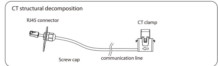
1. Insert the RJ45 connector of CT into the "RS485" port on the inverter, and screw down the screw cap tightly.
