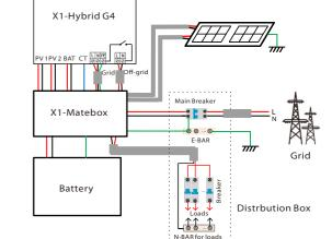
The Grid and Off-grid ports of X1-Hybrid G4 M series inverter have been connected, and the D series needs to be wired according to the following
