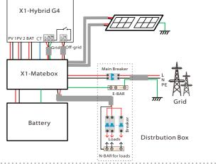
Diagram D: Neutral line and PE line are combined together, all loads connect to the Off-grid port; (Apply to Australia)
