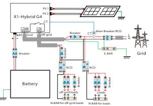
Diagram A: Neutral line and PE line are separated from each other, and
