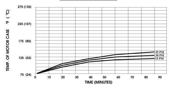
THIS GRAPH IS FOR USE AS A DESIGN GUIDE. IT IS BASED ON RUNNING CONTINUOUSLY WITH AN AMBIENT TEMPERATURE OF 70 F IN STILL AIR. THE THERMAL BREAKER WILL OPEN WHEN THE CASE TEMPERATURE REACHES 28%.
