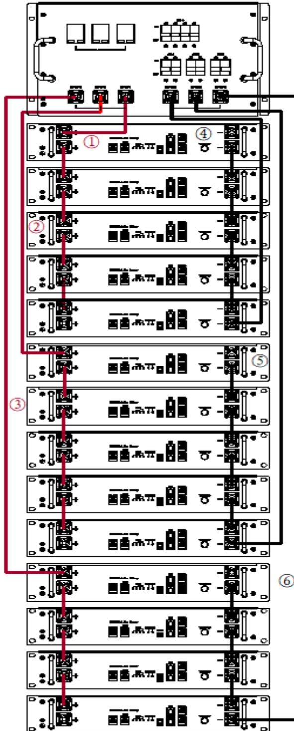
1#cable: 100mm    4#cable: 850mm
