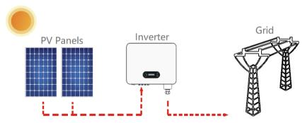
Figure 2-1 PV Grid-Tied System
