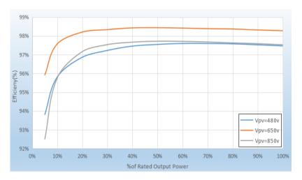
Figure 2-9 Power efficiency curve (take 20K for example)
