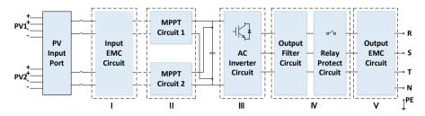
Figure 2-8 Schematic diagram
