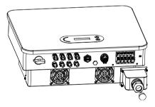
Figure 4-8 Removing AC waterproof cover diagram
