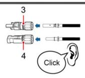
Figure 4-13 DC cable connection(3)
