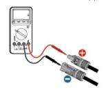
Figure 4-15 Use a multimeter to check the positive and negative electrodes
