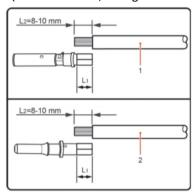
Figure 4-11 DC cable connection (1)
