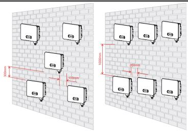
Figure 3-3 Clearance for multiple inverters
