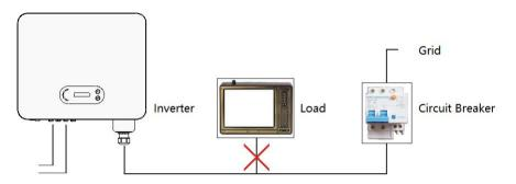
Figure 4-5 Incorrect connection between load and inverter
