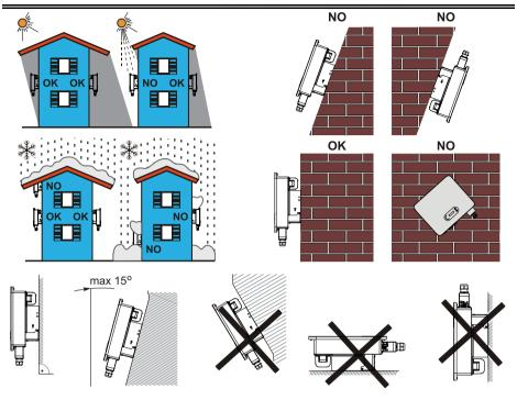
Figure 3-1Installation Position Selection
