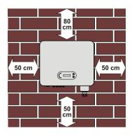
Figure 3-2Clearance for single inverter
