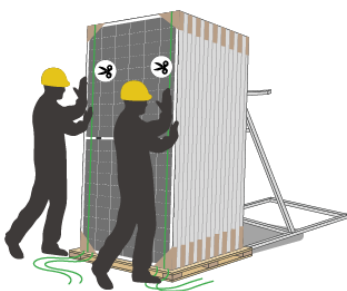
4) Place the stand supporter from the glass or backsheet side.
