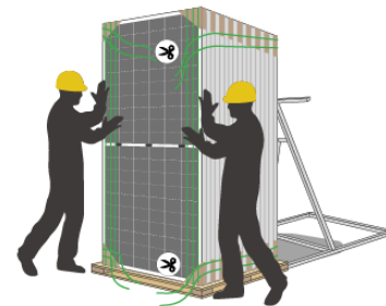
6) Cut off all the horizontal packing belts.
