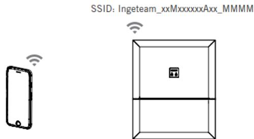
Once the device is connected to the Wi-Fi network, open the browser and enter IP address 169.254.1.1 to access the communication board management application.
