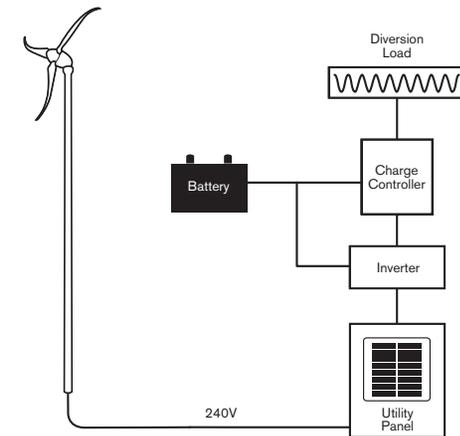
Battery Charging Block Diagram - with Xantrex Charge Controller with Diversion Load
