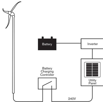
Battery Charging Controller Block Diagram
