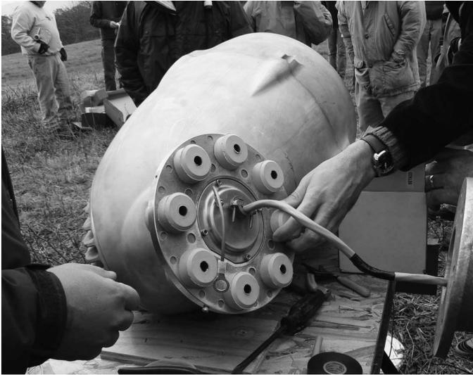
Fig. 9 Placing vibration isolators
