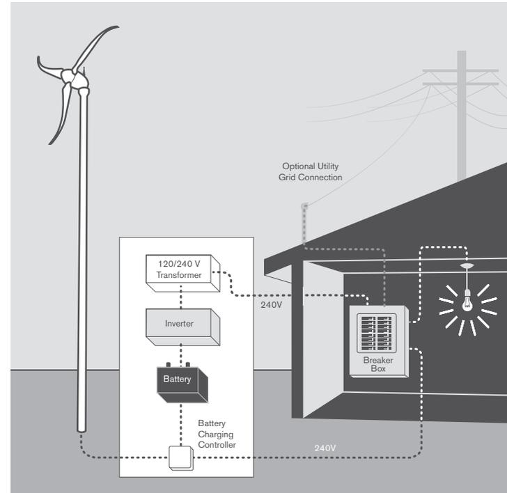
Fig.7- Battery Charging Option B
