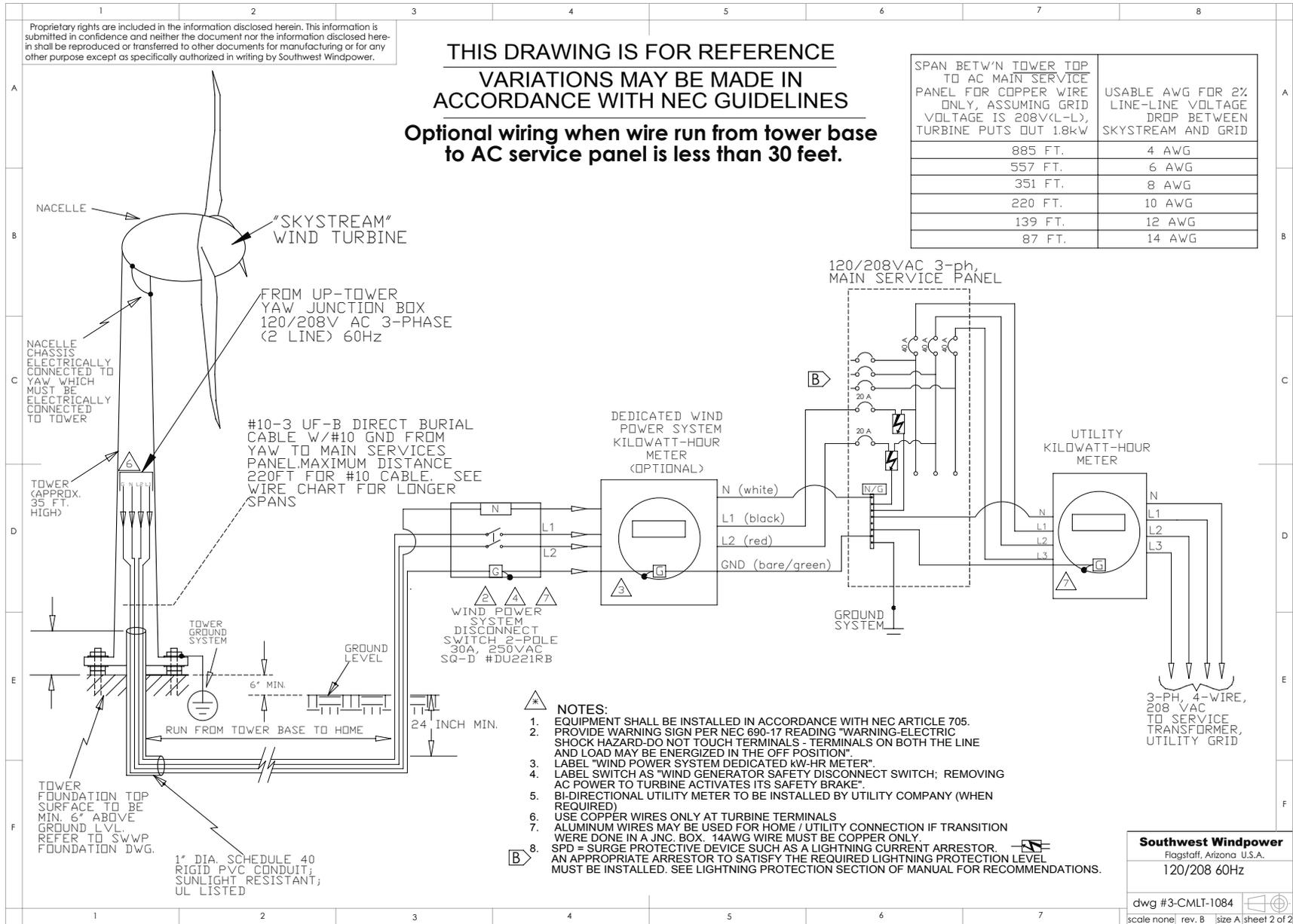
Fig. 5. Skystream Block Diagram
