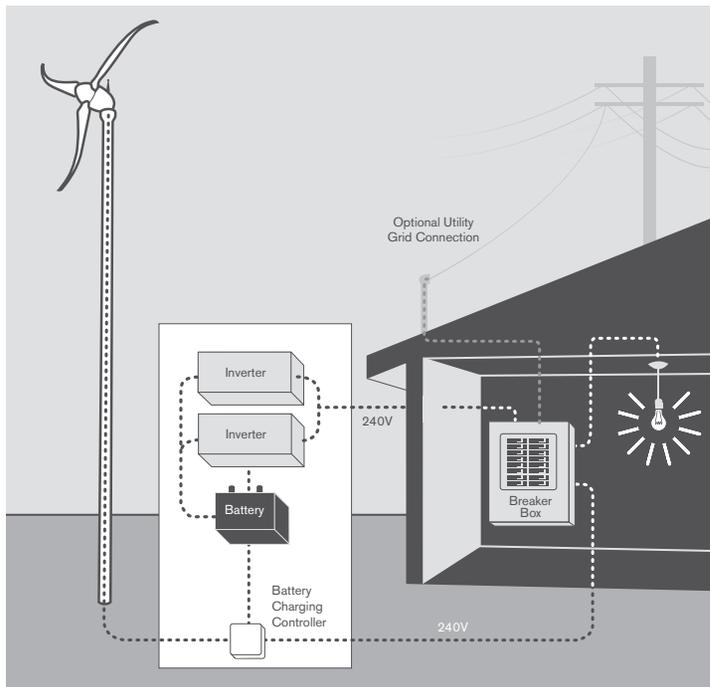
Fig. 6- Battery Charging Option A
