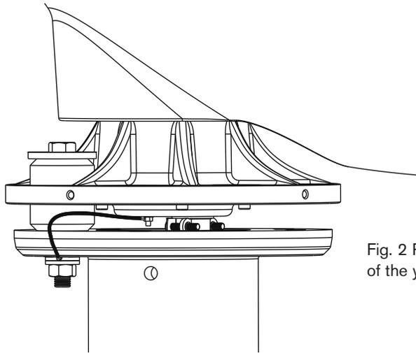
Fig. 2 Proper grounding of the yaw connection
