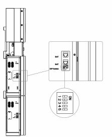
Step10 Open the front cover of the last battery and remove the DIP cover. Now set the DIP switch 2 to "on" mode and close the cover again.
