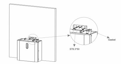
Step 5 To assemble the second (and all other) battery, repeat steps 6 and 7, respectively.
