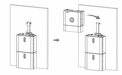
Step 7 Hang the inverter onto the mounting panels, adjust the entire system and ensure that the battery and the inverter have been securely hung onto the panels and brackets
