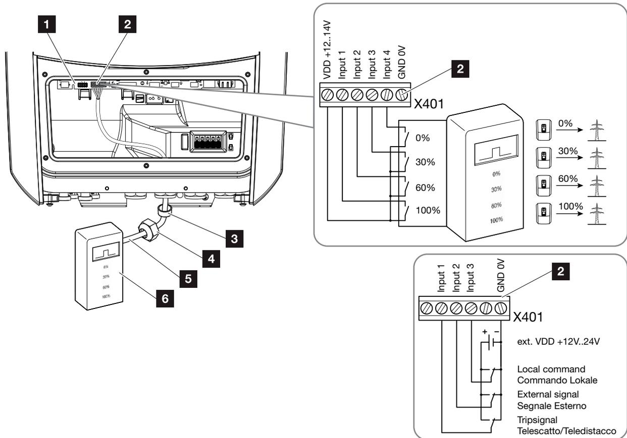
Fig. 31: Conexión del receptor de telemando centralizado
