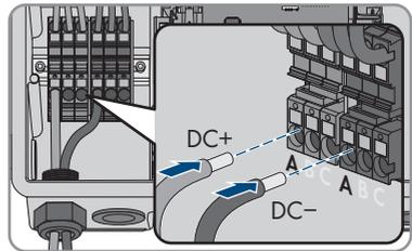
7. Ensure that the terminal points are allocated to the correct conductors.
