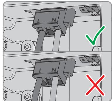
15. Ensure that the terminal points are allocated to the correct conductors.
