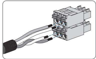
9. Make sure that the conductors are plugged into the terminal points tightly by pulling slightly on the conductors.
