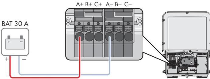
Figure 19: Overview for connection of one battery with a charging/discharging current limit of 30 A
