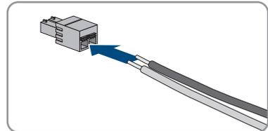
6. Stick the terminal block into the slot
