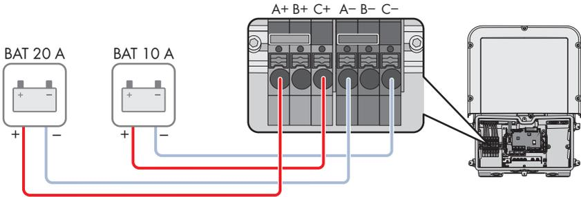
Figure 17: Overview for connection of two batteries with varying charging/discharging current limits
