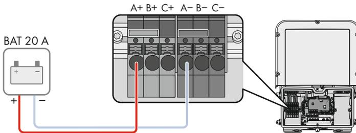
Figure 18: Overview for connection of one battery with a charging/discharging current limit of 20 A
