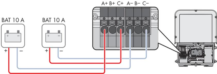
Figure 15: Overview for connection of two batteries with a charging/discharging current limit of 10 A each
