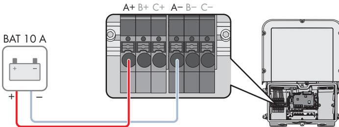
Figure 14: Overview for connection of one battery with a charging/discharging current limit of 10 A
