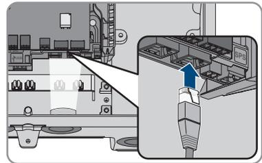
10. Ensure that the network connector is securely in place by pulling slightly on each cable.
