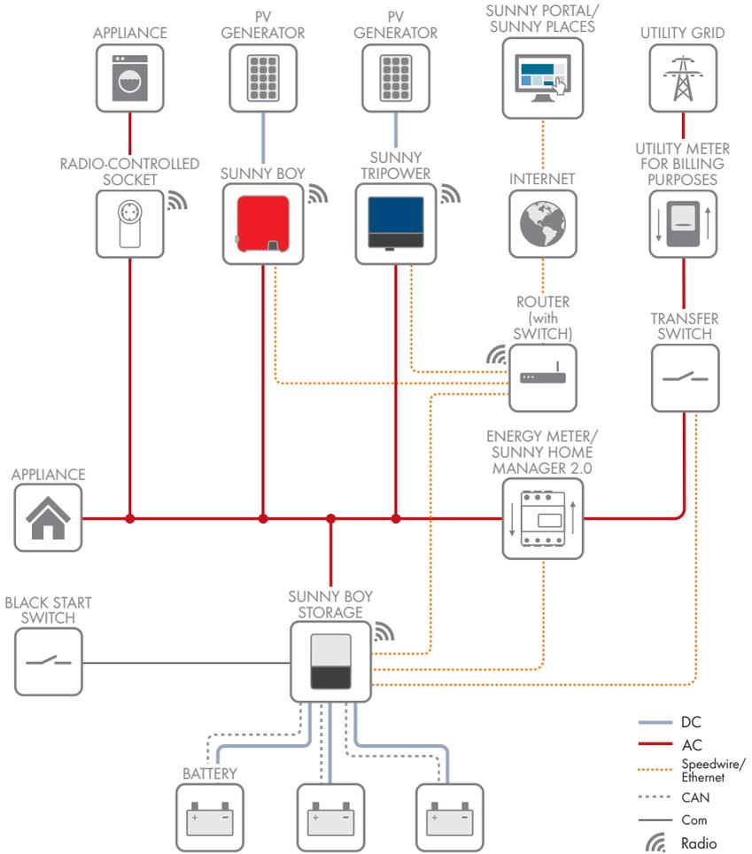
Figure 5: System design of a flexible storage system with battery-backup function (example) You can find a circuitry overview in the documentation of the automatic transfer switching device.
