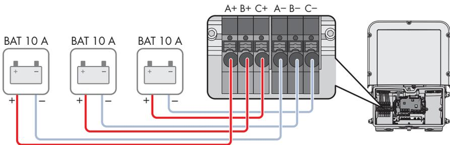
Figure 16: Overview for connection of three batteries with a charging/discharging current limit of 10 A each
