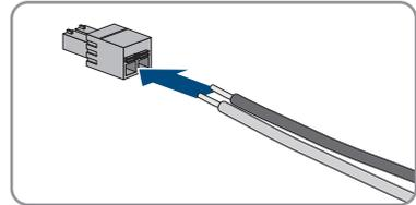
6. Stick the terminal block into the slot
