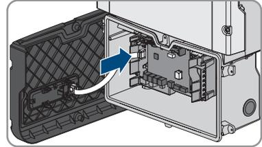
2. Ensure that the ribbon cable is securely plugged into the sockets at both ends.
