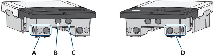
Figure 12: Enclosure openings at the bottom of the inverter
