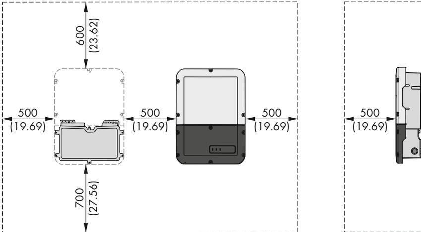
Figure 11: Recommended clearances (Dimensions in mm)
