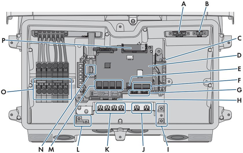
Figure 13: Connection areas in the interior of the inverter
