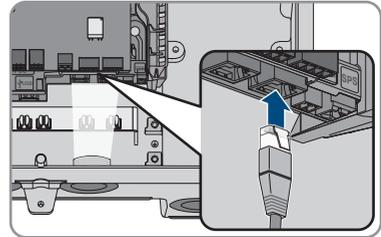
9. Ensure that the network connector is securely in place by pulling slightly on each cable.
